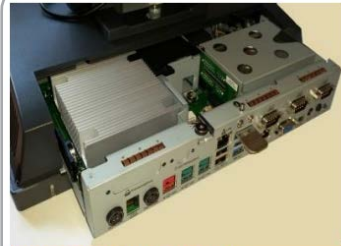
Slide in / out motherboard
